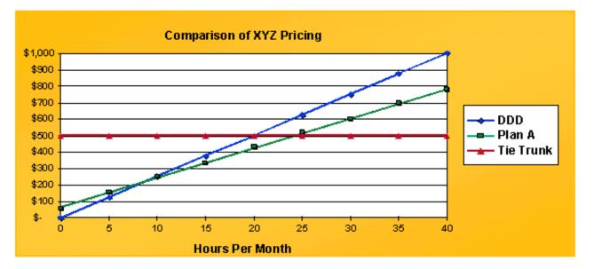
The Tie Trunk, represented by the red line, is a straight line at \$500. DDD is a linear line that starts at 0. To optimize costs, the goal is to stay below the curve. The cross-over points between the different plans occur at 8.57 hours between DDD and Plan A,
